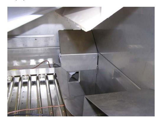
Feed the bin probe from the upper machine, through one of the holes in the upper machine condensing unit pan and position in one of the holes in the lower ice machine condensing unit pan and adjust as required (illustration below).
